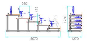
Retractable tribune with liftable and foldable armchair over the grandstand
