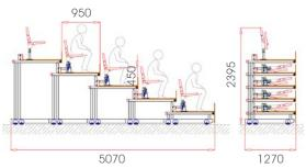
Telescopic tribune with automatic polypropylene foldable and liftable seat front of the grandstand.
