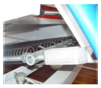
The basket has springs for its manual lifting with safety telescopic bar anchored to the front and rear pole with safety pins which have three stops, one for basketball game, one for mini basketball game and another for transportation and storage.
