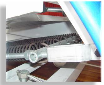
The basket has springs for its manual lifting with safety telescopic bar anchored to the front and rear pole with safety pins which have three stops, one for basketball game, one for mini basketball game and another for transportation and storage
