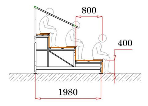
Fixed tribunes assembled through Steel screws with a minimum platform of 800mm. With wooden bench seat (DM) attached to the top of the platform through screws. Legs fixed on the ground to ensure complete fixation. It is supplied by pieces and they are assembled through steel screws.
