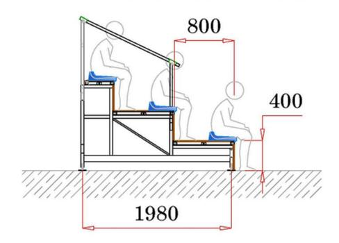
Fixed tribunes assembled through Steel screws with a minimum platform of 800mm. With TP SPORTS seats, S90-SG attached to the top of the platform through screws. Legs fixed on the ground to ensure complete fixation. It is supplied by pieces and they are assembled through steel screws.
