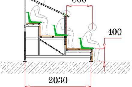
Fixed tribunes assembled through Steel screws with a minimum platform of 800mm. With TP SPORTS seats, S97-SG attached to the top of the platform through screws. Legs fixed on the ground to ensure complete fixation. It is supplied by pieces and they are assembled through steel screws.
