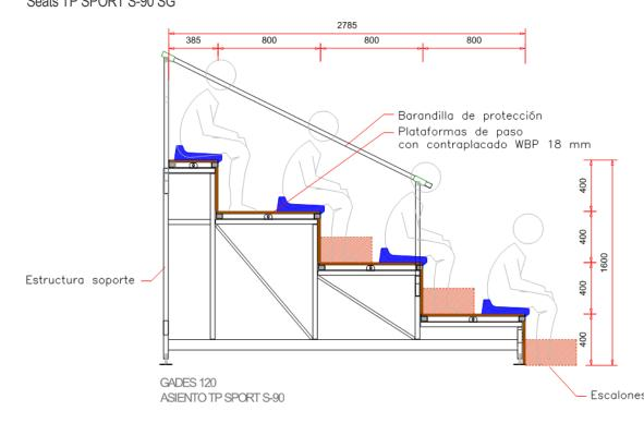
Removable tribune assembled through steel screws with a minimum platform of 800mm. Prepared to fit individual seats model TP SPORT S-90 SG on the top of the platform through screws. It is supplied by pieces and they are assembled through steel screws.
