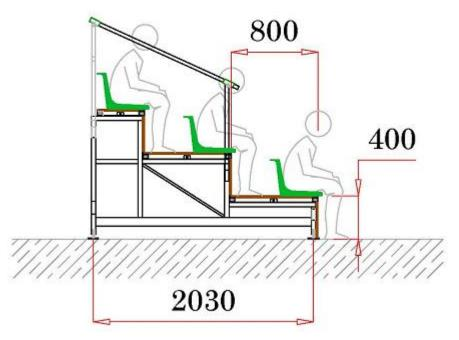
Removable tribune assembled through steel screws with a minimum platform of 800mm. Prepared to fit individual seats model TP SPORT B-92 SG on the top of the platform through screws. It is supplied by pieces and they are assembled through steel screws.
